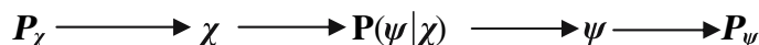
Figure 1. The “geometric” AO→MO information channel defined by the spinless conditional probabilities of Equation (1). The AO probabilities \mathbf{P}_\chi (Equation (3)) determine the distribution of the input signals, in the channel “source,” while the MO probabilities \mathbf{P}_\psi = \mathbf{P}_\chi \mathbf{P}(\psi|\chi) (Equation (3)) define the associated probabilities of the output signals, in the channel “receiver.” The input probabilities reflect the initial (promolecular) occupations N of AO in the non-bonded atoms.
